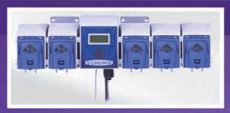
V-Line OPL Laundry System - Is the perfect on-premise laundry system for facilities where value and flexibility are critical but performance must be second to none. V-Line features a modular design to accommodate from 1 to 6 pumps and uses the proven performance of DEMA's standard Quick Change Pump at 16 ounces (475 ml) per minute or the Large Blue QC Pump for 50 ounces (1500 ml) per minute Designed to be fast and convenient for OPL installations.
